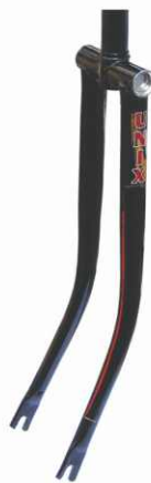
UG-14 RL. TYPE For Wheel Size 28 x 1.1/2, Tubular Crown W/BCP Thimbles Column dia : 25.4 x 26/24 TPI.
