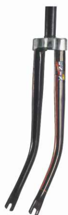
UG-17 PH. TYPE For Wheel Size 22" / 24" 28 x 1.1/2", Box Crown, 25.4 x 24 TPI Column Length to order.
