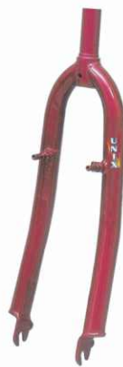
UG-12 MTB TYPE (With Pivots) For Wheel Size 26 x 2.125" Unicrown 24 TPI, Suitable for Cantilever Brakes Flamboyant/Metallic Laser Colours.
