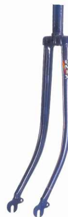
UG-15 SLR TYPE For Wheel Size 26 x 1.3/8", Column dia : 25.4 x 24 TPI Pressed Sheet Ends.
