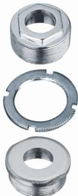
UG-313 B.B CUP ITALIAN TYPE Set of 3 Thread : 35mm x 24 TPI, BSCY RH+RH 34.8 & 36mm Also Available
