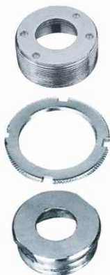
UG-312 B.B. CUP PH. TYPE Set of 3, RH & LH Threads Thread : 34.8 x 24 TPI or 26 TPI, BSCY RH+LH 35x1mm or RH+RH 35 x 1mm
